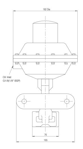
Weight (caliper and thruster) - 5.5kg (thruster only) - 4.0kg Volume displacement of thruster at 4mm retraction = 5ml.
