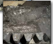
Severe damage on non-genuine friction disc
