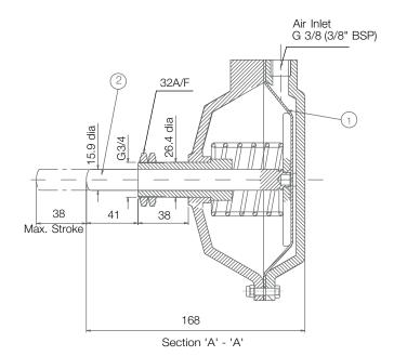
This range of pneumatically operated brakes uses dry and filtered compressed air at pressures up to 7 bar. Pneumatic brakes require a control valve which may be operated either manually, or by pneumatic or electric signal.
