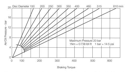
The ratings shown on the above graph are based on fully bedded-in pads.
