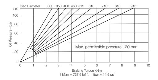
Brake Perfomance of T20 Disc Brake Caliper
